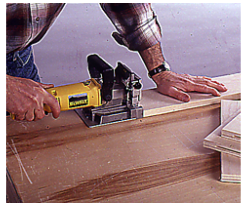
6--To cut plate slots in the end of plywood parts, hold the workpiece down and slide the plate joiner on the bench.
