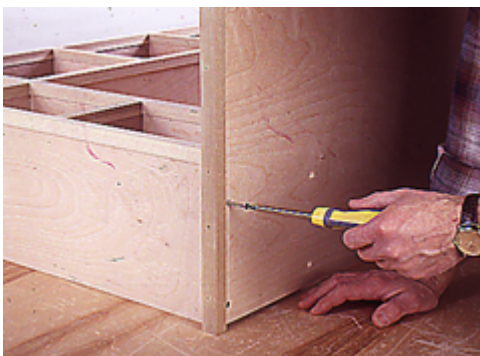
17--Fasten the storage shelf to the desktop by driving SCREWS through the desktop and into the shelf sides.
