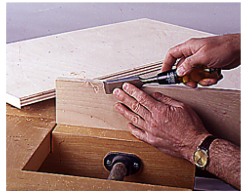
3--Use a chisel to trim the birch veneer tape to width. Cut from the opposite direction if the tape tears out.
