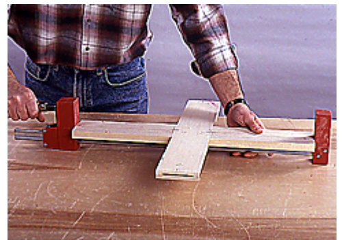
9--Begin the assembly of the open grid by gluing and clamping together the center horizontal and vertical pieces.
