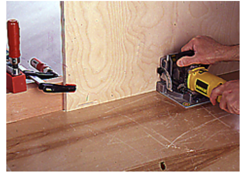
4--To cut joining plate slots on the panel's face, clamp the panel upright, and slide the plate joiner on the work surface.
