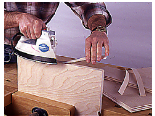
2--Use an iron to apply heat to the birch veneer tape. The banding has heat-sensitive adhesive on its back.
