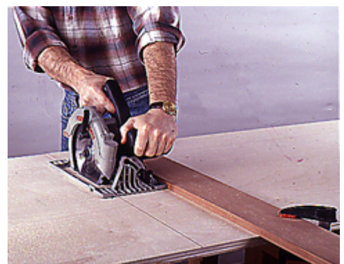
1--To cut the plywood desk parts to size, use a circular saw guided by a straightedge clamped to the panel's face.
